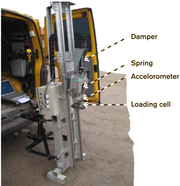
▲ The Orono Biomechanical Surface Tester simulate the impact of a horse’s leg on the ground. The machine is mounted at the back of a van or truck of sufficient weight, for ease of transport between and on arenas, and is supported by a frame, which is placed on the ground for stability during testing.
