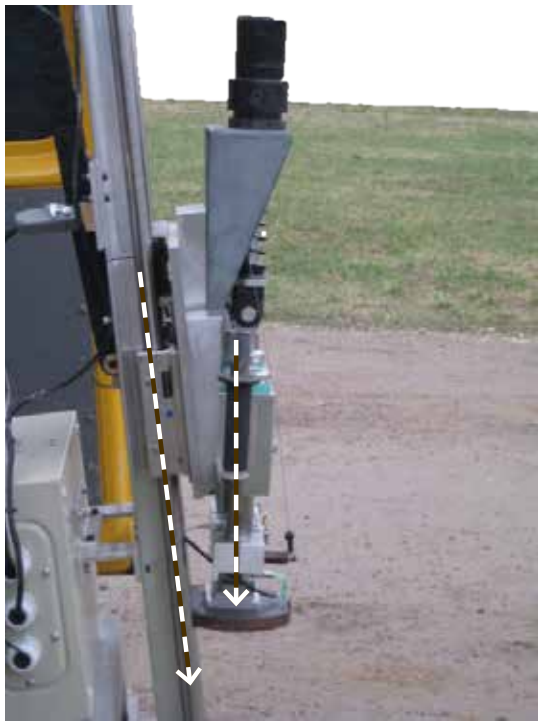
▲ The metal “hoof” is mounted beneath a heavy weight, which is dropped to the ground between two guide rails. The rails have different angles, which mimics the motion of the early landing/touchdown phase, as a simultaneous downward motion and forward slide of the ‘hoof’ occurs when it contacts the ground.
